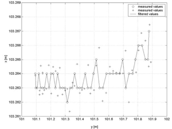
**Figure 13:** Measured, predicted and filtered values of reflector position at  $q = 10$
