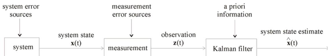
**Figure 2:** Block diagram depicting system, measurement and estimator (Gelb, 1974)
