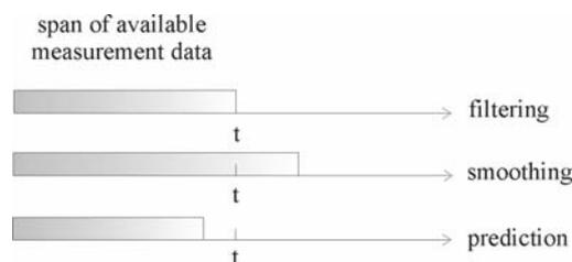
**Figure 1:** Three types of estimation problems; estimate desired at time  $t$  (Gelb, 1974)
