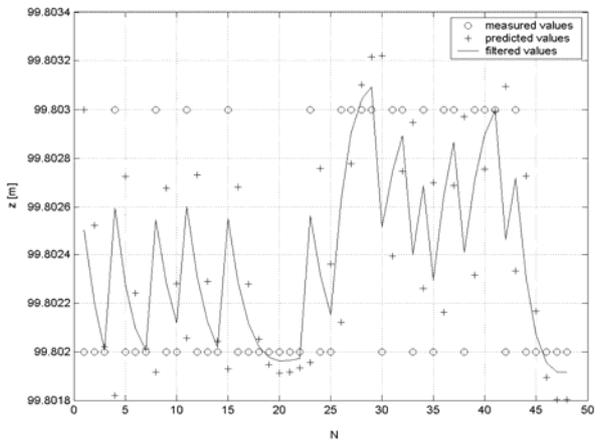
**Figure 7:** Measured, predicted and filtered values of position components of the reflector for  $q = 0.00001$
