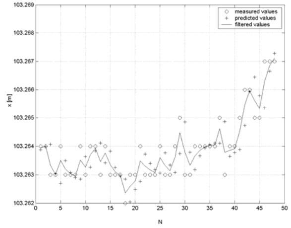
**Figure 7:** Measured, predicted and filtered values of position components of the reflector for  $q = 0.00001$
