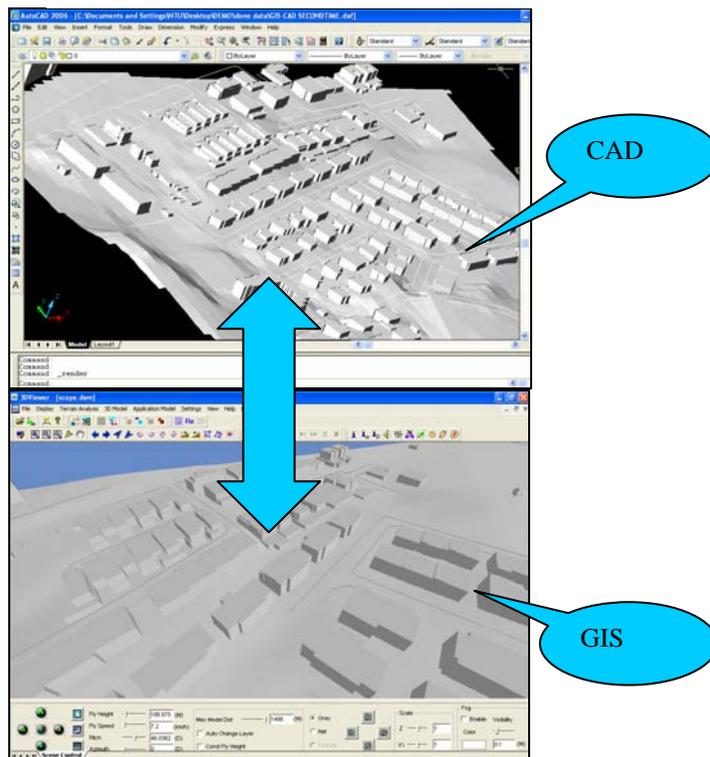
**Fig. 6.** Model translation between AutoCAD and VGEIS
