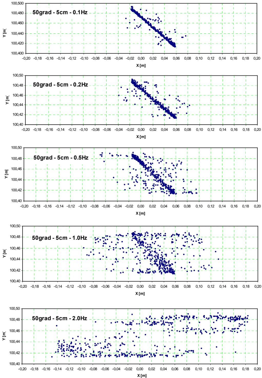
**Figure 6:** Recorded coordinates of the prism location for a 50 grad twist angle, 5 cm amplitude and for a frequency bandwidth ranging from 0.1 Hz to 2 Hz.
