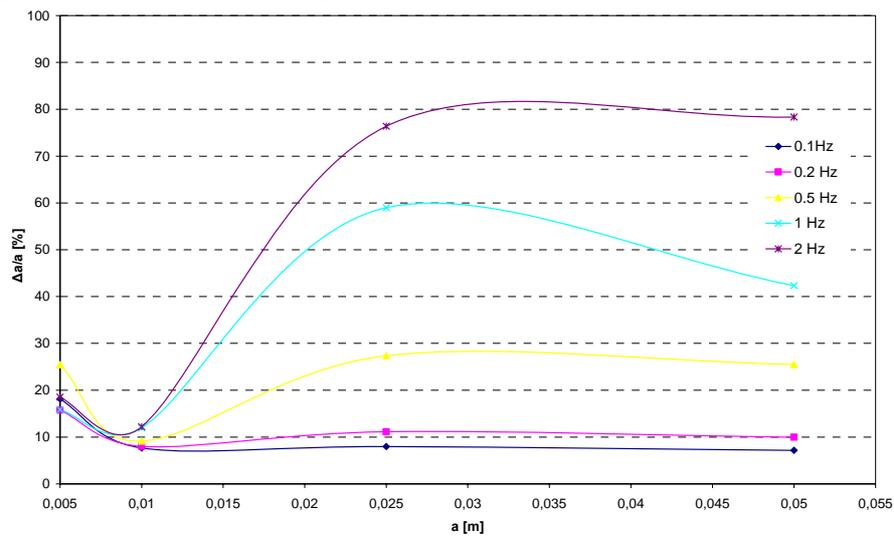
**Figure 5:** Percentage  $\Delta a/a$  (%) of the mean differences between the nominal and the observed amplitude as a function of the nominal frequency and the twist angle.
