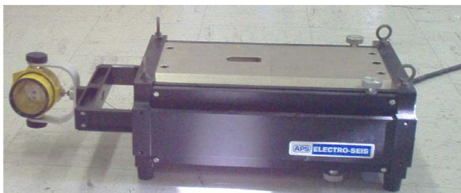
**Figure 1:** The electrodynamic shaker with the circular prism mounted on the oscillating arm.
