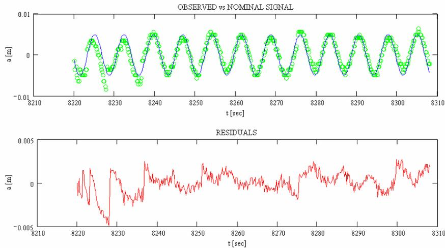
**Figure 4:** Recorded time series by the total station (circles) superimposed by the nominal signal (continuous line) [top]. Residual values [bottom]
