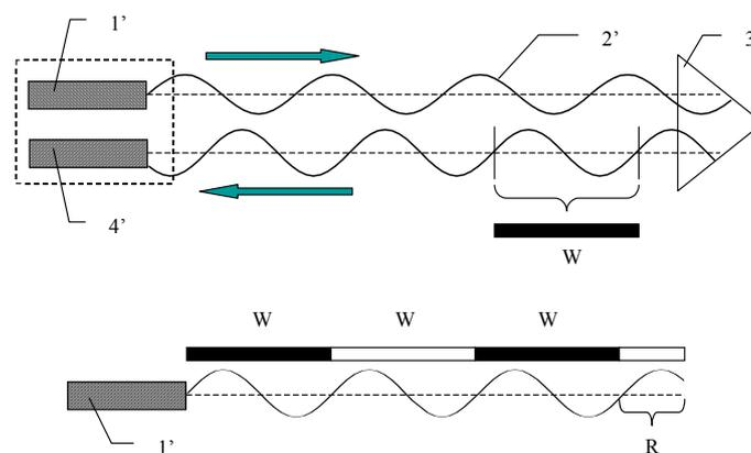
**Figure 6:** The principle of the phase measuring method
