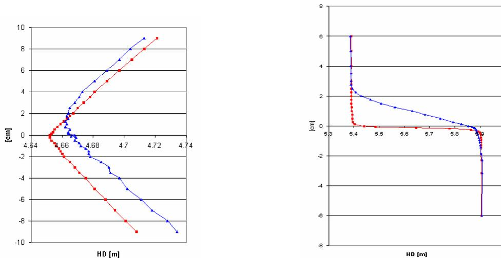
**Figure 11:** Corner measurements using Leica's EDM compared with a time-of-flight EDM
