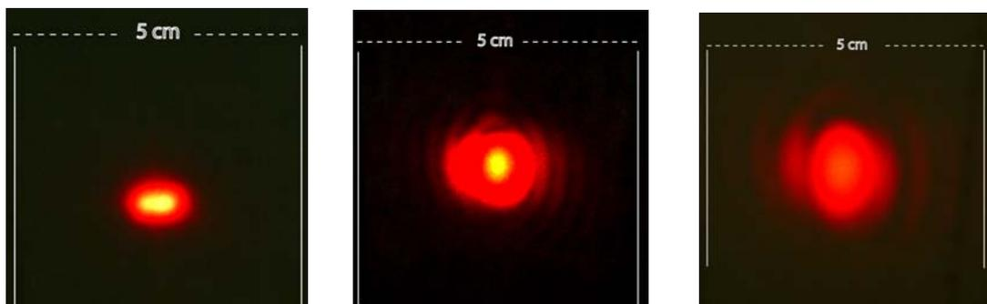
**Figure 10:** Leica's laser spot size at distance: 5, 35, and 55 m
