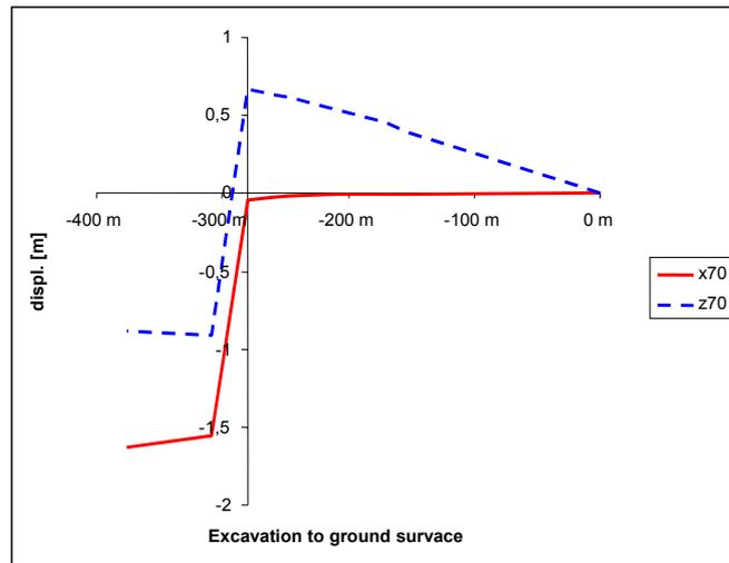
**Figure 9:** Prediction of a local failure event in history point 70
