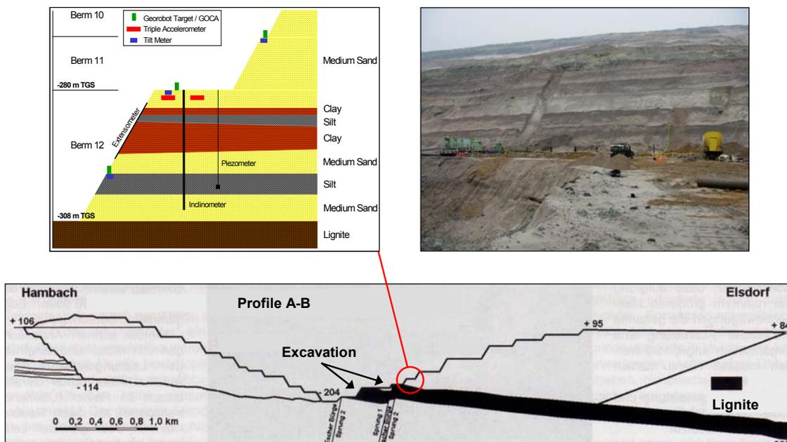
**Figure 3:** Test-slope with installed geotechnical monitoring system in opencast mine
