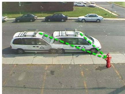
**Figure 5:** Single Camera Parallax
