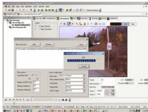
**Figure 8:** Automated Sign Detection
