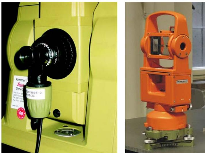
**Fig. 2:** Autocollimation-eyepiece from Leica Geosystems and Autocollimation-mirror GAPI from Wild Heerbrugg.
