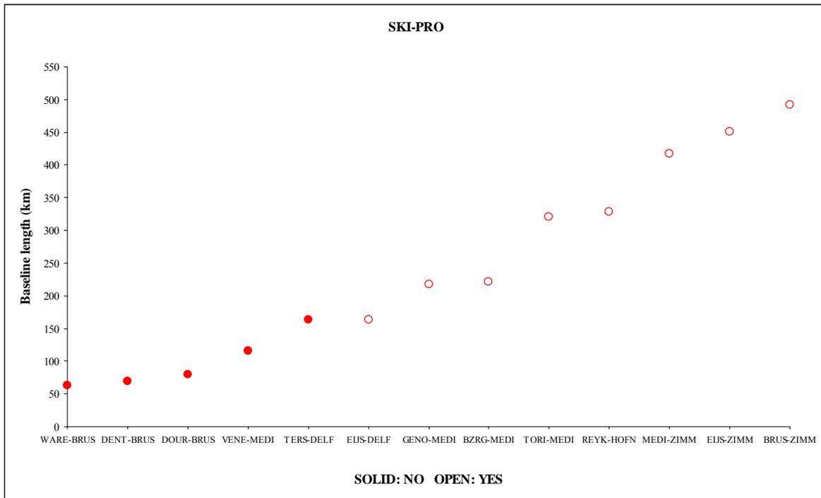
**Figure 6b.** Comparison between the mean distances with their rms and EPN values for all the tested baselines using SKI-PRO for 1-sigma confidence region. The solid circle means that the true distance is outside the confidence region of mean value (No). The open circle means the opposite (Yes).
