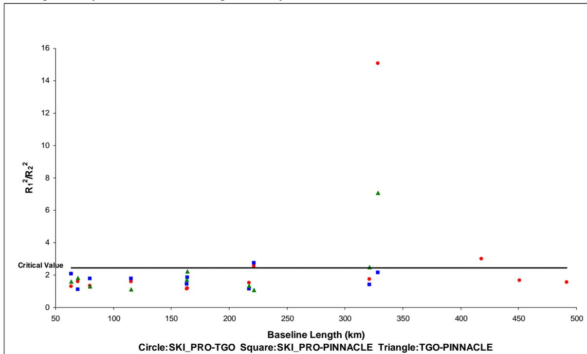
**Figure 3.** Repeatability compatibility test as a function of baseline length between pairs of GPS software
