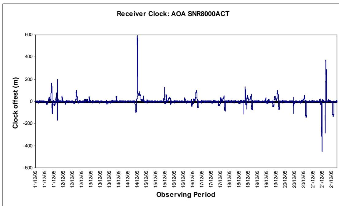
**Figure 8a.** The clock offset of Reykjavik station receiver for the test period.
