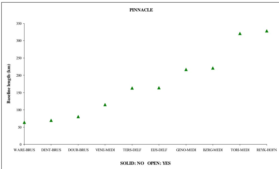
**Figure 5a.** Comparison between the weighted mean distances with their rms and EPN values for all the tested baselines using Pinnacle for 1-sigma confidence region. The solid triangle means that the true distance is outside the confidence region of the weighted mean (No). The open triangle means the opposite (Yes).
