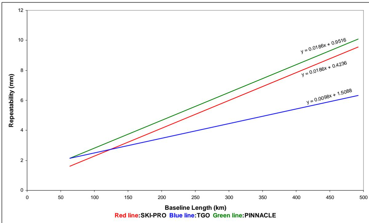
**Figure 2.** Best fitting lines on repeatability values according to baseline lengths for the test GPS software packages
