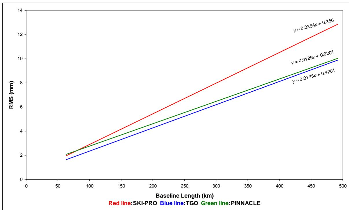
**Figure 4.** Best fitting lines on the derived rms values versus baseline lengths for the test GPS software's
