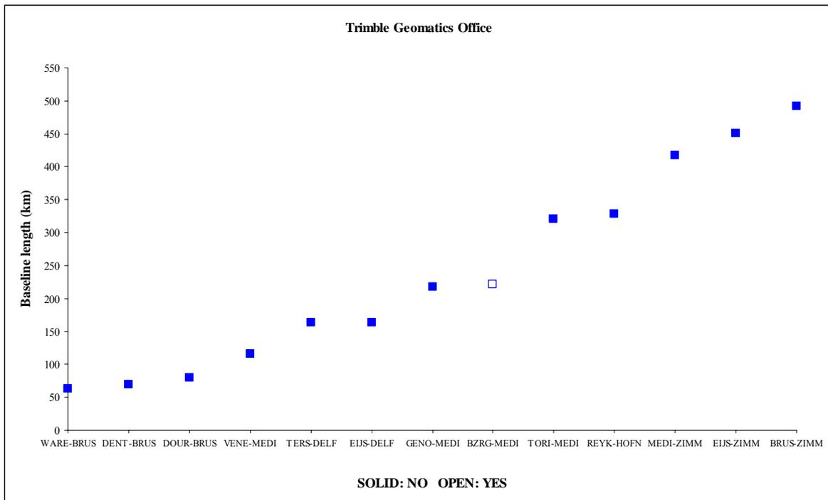
**Figure 7a.** Comparison between the weighted mean distances with their rms and EPN values for all the tested baselines using TGO for 1-sigma confidence region. The solid square means that the true distance is outside the confidence region of weighted mean (No). The open square means the opposite (Yes).
