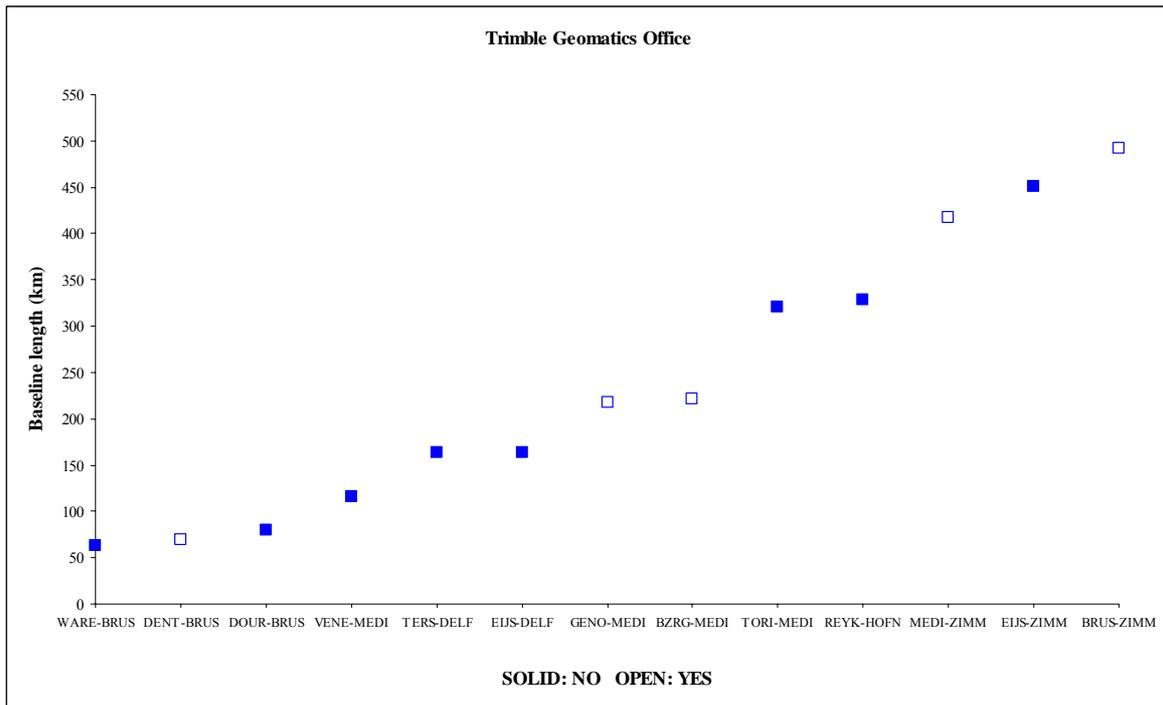
**Figure 7b.** Comparison between the mean distances with their rms and EPN values for all the tested baselines using TGO for 1-sigma confidence region. The solid squares mean that the true distance is outside the confidence region of mean value (No). The open square means the opposite (Yes).
