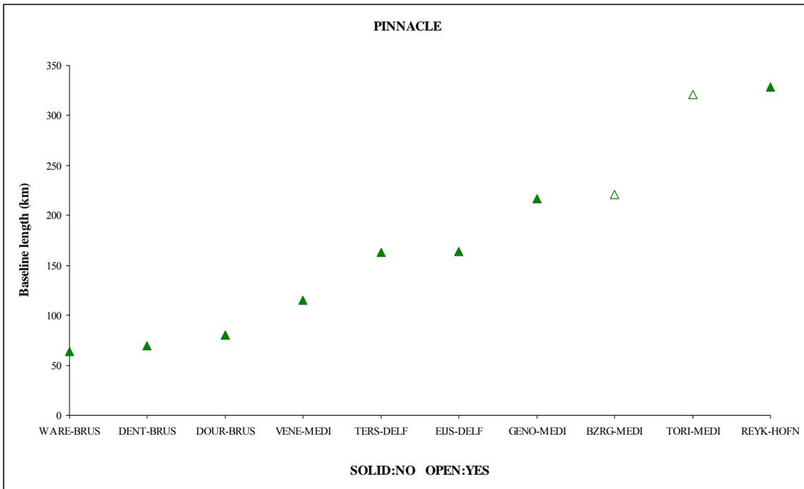
**Figure 5b.** Comparison between the mean distances with their rms and EPN values for all the tested baselines using Pinnacle for 1-sigma confidence region. The solid triangle means that the true distance is outside the confidence region of mean value (No). The open triangle means the opposite (Yes).
