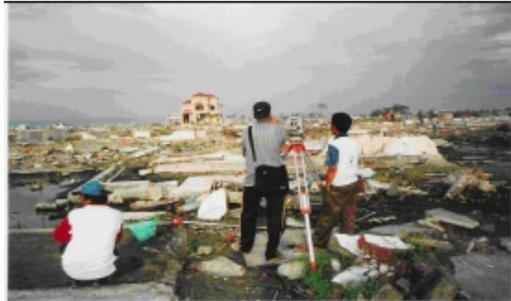
**Figure 7(b).** Example of parcel boundary reconstruction in Aceh with Total Station
