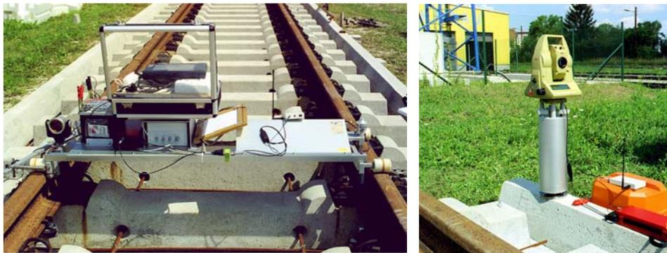
**Fig. 10:** Track measuring vehicle and tachymeter on special pillar
