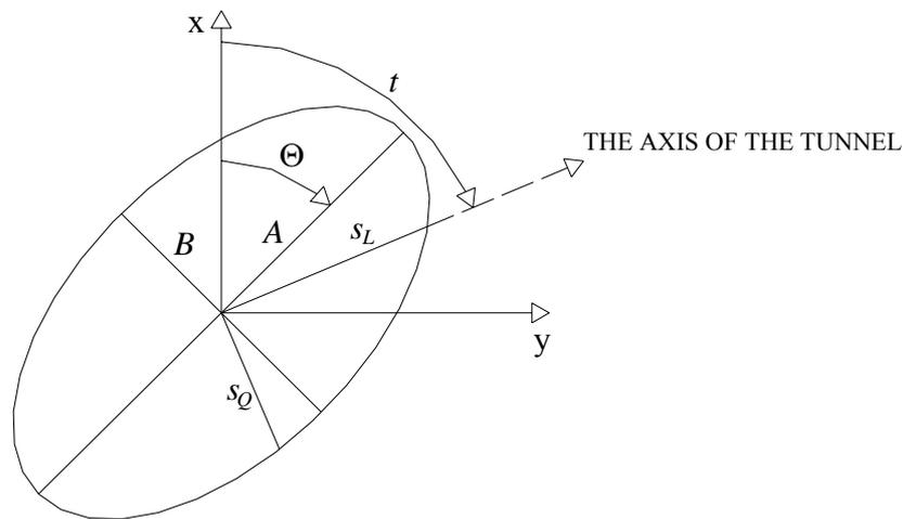
**Fig. 1.** Longitudinal and transverse deviation of tunnel cutting point.
