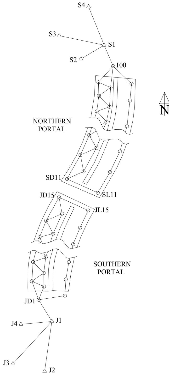
**Fig. 3.** Sketch of the underground geodetic basis of the tunnel "Mala Kapela".
