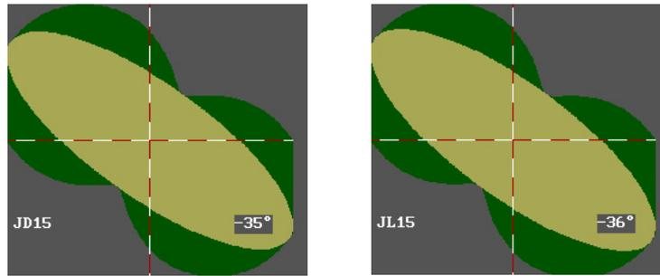
**Fig. 5.** Error ellipse and foot curves of the last network points from the cutting was made on the southern tunnel portal (scale unit = 1 cm).
