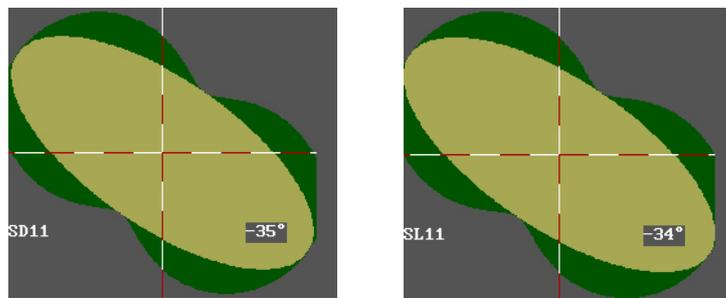
**Fig. 4.** Error ellipses and foot curves of the last network points from which the cutting was made on the northern tunnel portal (scale unit = 1 cm).
