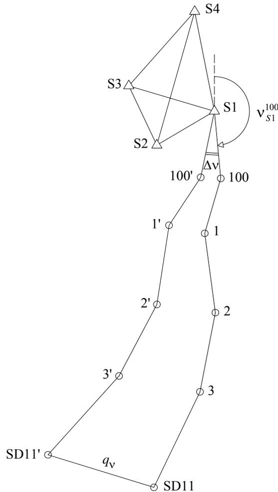
**Fig. 2.** Influence of the error of the initial bearing angle on transverse deviation in tunnel cutting.
