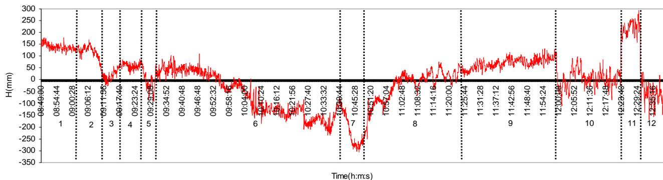
**Figure 3** Time series of Bosphorus Bridge responses under different loads.
