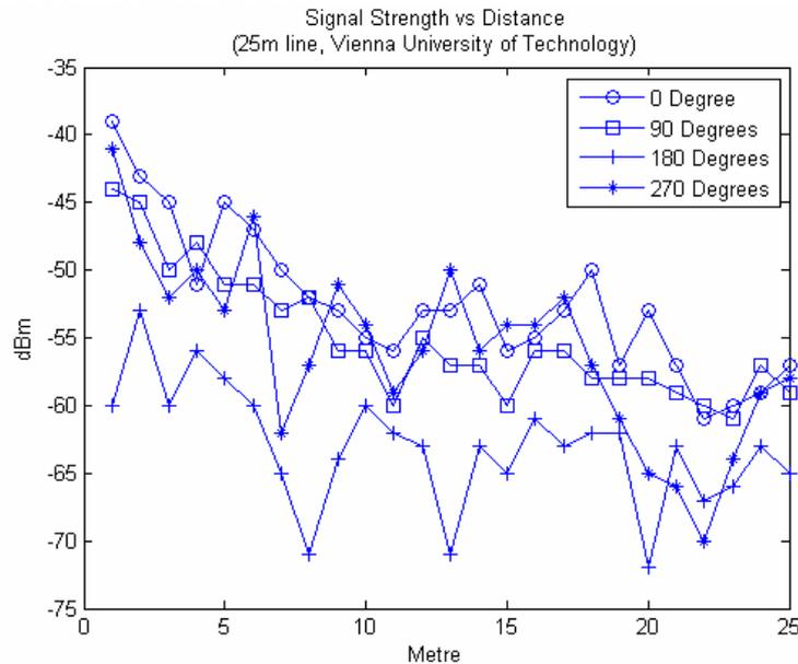
**Figure 5 (a):** Test result of signal strength vs distance over a 25 metre baseline at TU Vienna
