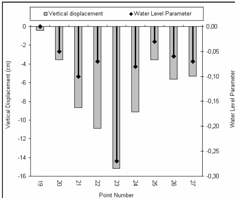
**Figure 3.** Relationship between vertical displacements and water level parameter
