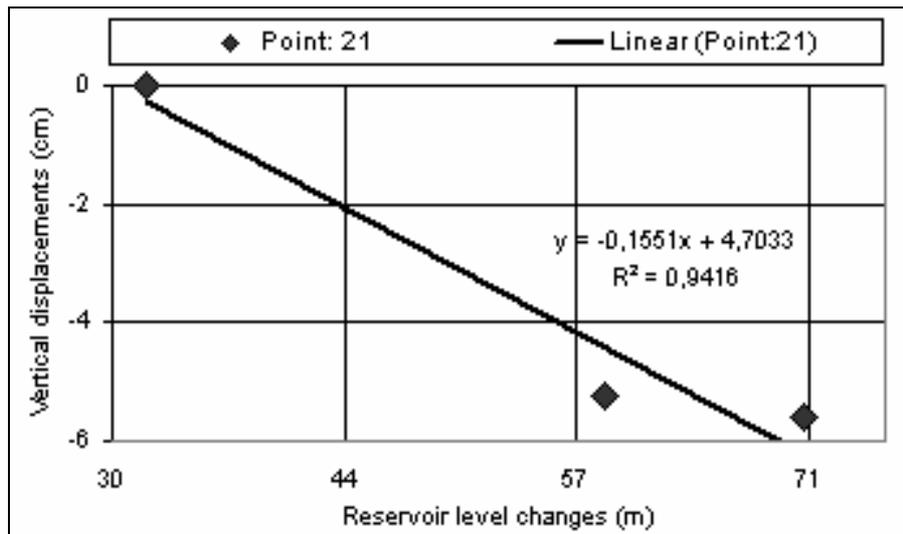
**Figure 2.** Relationship between reservoir level rising and vertical displacements at point 21
