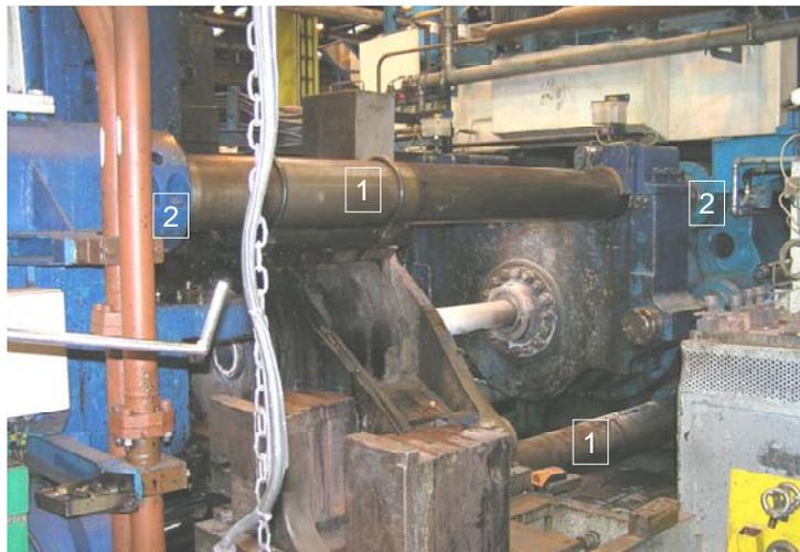
**Fig. 6.** The tie rods (1) and the nuts (2) - by courtesy of ALCOA KÖFÉM
