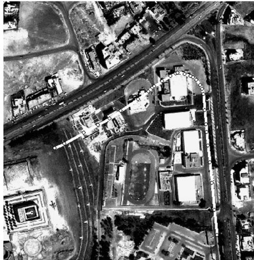
**Figure 10:** Overlay of IKONOS with field data before registration
