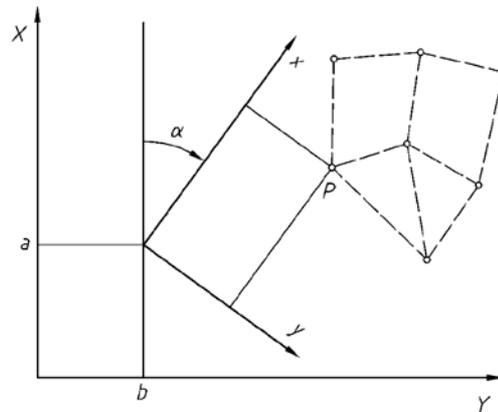
**Fig. 3:** Graphical explanation of a 2D similarity transformation (see: DIN 18709-4, 2005)
