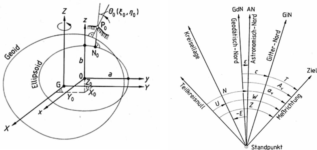
Fig. 2: Geodetic datum and measurement of directions with a gyro (see: DIN 18709-1, 1995)
