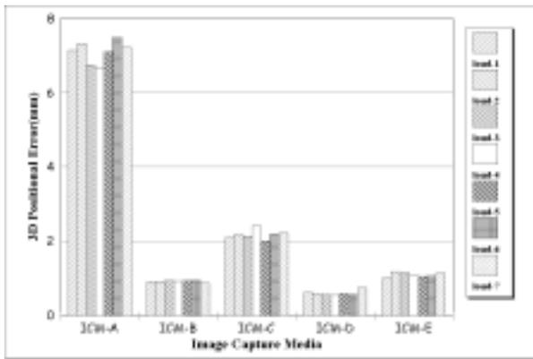
The case of ICM-D analyzed by using the image of DCS200 and the image of 35 film showed relatively most improved standard error of vertical direction of 0.1816, and the case of ICM-B and ICM-E interpreted by scanning film image showed the standard error of the direction of Y
