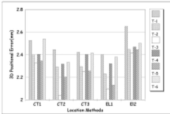
Fig. 6 3-dimensional Position Error by the Method of Image Segmentation which is based on the Location Method camcoders. And, out of centroid location methods, CT2 method which used greylevel value as weight showed more improved accuracy. The result interpreted by applying location EL(II) method showed the accuracy distribution which is low relatively in
