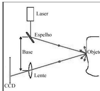
Figure 06: Scanner based on the principle of triangulation
