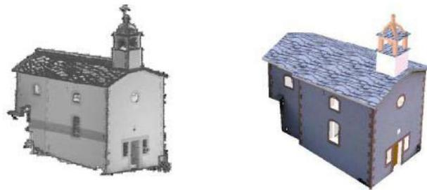
Figure 13 and 14: Point Cloud and 3D model of the Chapel "Neubrueck"
