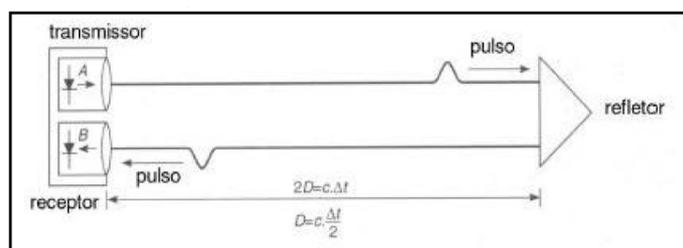
Figure 04: Principle of scanning time-of-flight (time interval)
