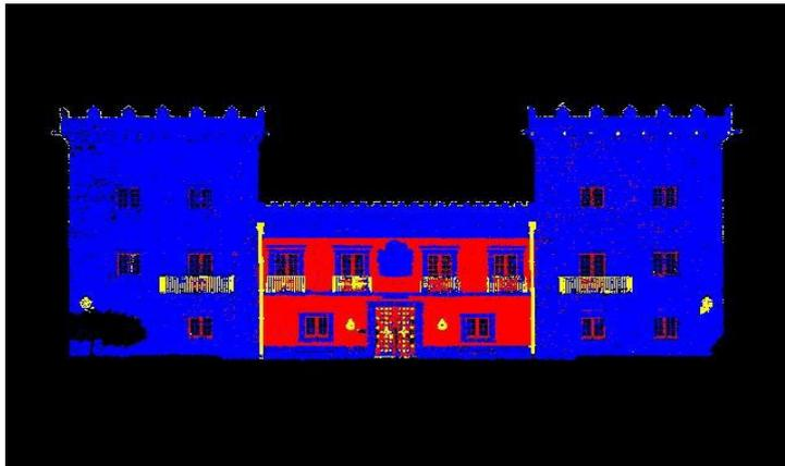
Figure 10: Facade classified (in blue granite, white wall in red and yellow iron)
