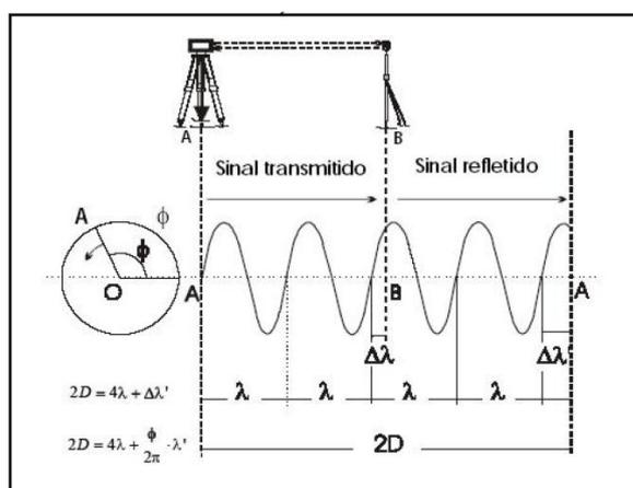
Figure 05: Determination of distances by road double
