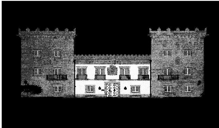
Figure 09: Result of cleaning performed on the point cloud
